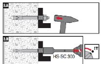
Check setting and apply the required torque
