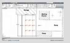
**Hilti Point Creator:** A tool used to extract point coordinates from 2D or 3D BIM/CAD drawings from AutoCAD or other BIM applications. These point coordinates and attributes can be easily transferred to Hilti POS 150 and POS 180 robotic total stations.
