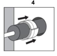
Install Hilti Firestop Bandage CFS-B on both sides within the opening in a depth of 62.5 mm.
