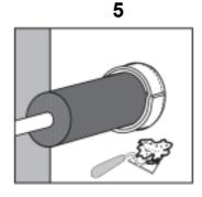
Close the remaining gap with mortar or gypsum.
