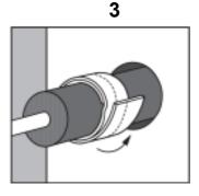
Wrap Hilti Firestop Bandage CFS-B around the insulation. Secure the bandage with steel bands or wire (≥ 0.7mm)
