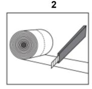
Cut Hilti Firestop Bandage CFS-B to fit the outside diameter of the insulation. Consider the number of 2 layers.
