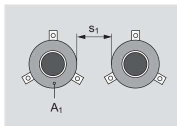
**Collars to be fixed** with hooks (F) and M8 metal anchors. In high density rigid walls alternatively metal anchors with minimum Ø 8 mm may be used. For minimum number of hooks see 1.1.
