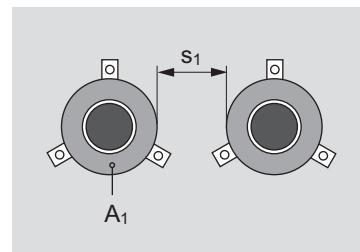
Pipes shall be supported at maximum 200 mm (pipes according to 2.3.1), at maximum 300 mm (all others) away from the upper face of the floor construction.
