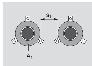
**Collars to be fixed** with hooks (F) and threaded rods M8 through the wall and nuts on both sides of the wall. In high density rigid walls alternatively metal anchors with minimum Ø 8 mm may be used.
