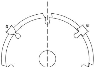
The width of the slot G between the segments must not exceed 10 mm ( $\frac{3}{8}$ "'). The thickness of the disc must not exceed 3.5 mm ( $\frac{1}{8}$ "').
