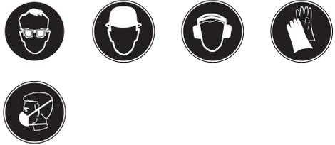
**The user and any other persons in the vicinity must wear ANSI Z87.1-approved eye protection, a hard hat, ear protection, protective gloves and breathing protection while the machine is in use.**
