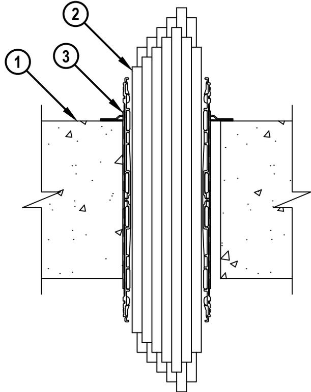
1. CONCRETE FLOOR OR WALL ASSEMBLY (2-HR. FIRE-RATING) :
