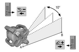
1. Use the visual sighting method on the head to line up the vertical axis of the rotating laser.
