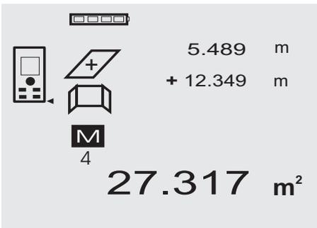
The tool saves measurements and the results of calculations continuously while in operation. A total of up to 30 values, including graphic symbols, are saved in this way. The complete set of information displayed is saved in the following situations:
