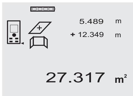
The painter’s area function is used, for example, to determine the surface area of the walls in a room. This is done by determining the total length of all walls and multiplying this figure by the height of the room.
