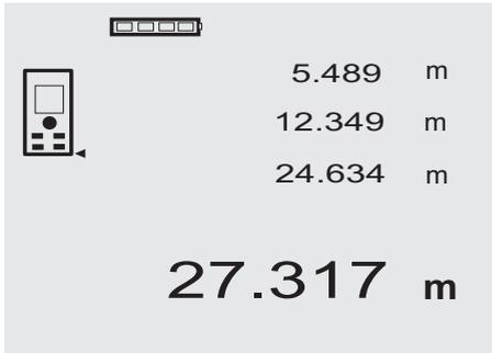
If several distance measurements have been taken, up to 3 previous measurements are shown in the intermediate result lines in the standard display, i.e. in total, the 4 previous measurements are shown and saved. The last measurement taken is shown in the lowest line of the display.
