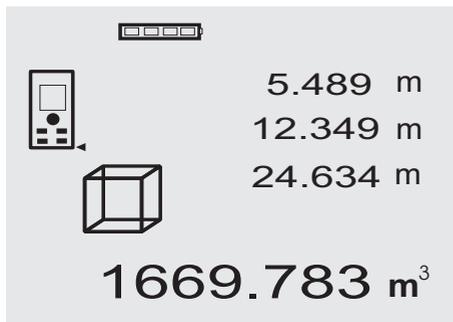
Each step of the volume measurement operation is indicated graphically in the display. For example, to determine the volume of a room, proceed as follows:
