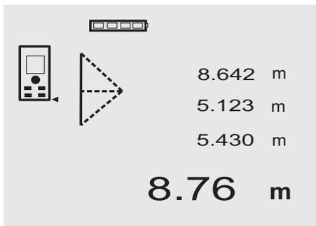
Follow the symbols in the display. The blinking side of the triangle indicates the measurement to be taken. When the 3 required distances have been measured, the result is then calculated and shown in the result line at the bottom of the display.
