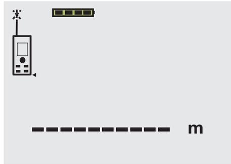
Aim at the target. Press the “Measure” button once again to measure the distance. The result usually appears in the result line in less than a second and the laser beam then switches off.
