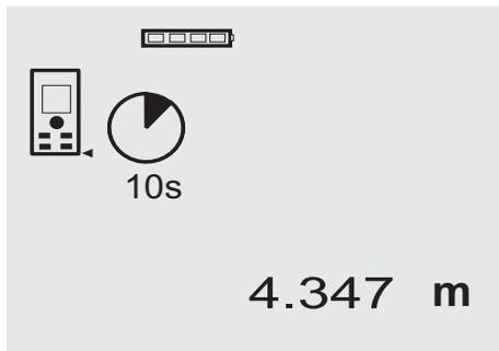
The timer function works like the self-timer on a camera. The "Plus" and "Minus" buttons can be used to adjust the timer interval to one of the three settings: 5, 10 or 20 seconds. To activate the timer, press the "Measure" button. To stop the timer, press the C-button. A beep sound is emitted every second up to about 4 seconds before the timer triggers the tool. The last 4 seconds are counted down by a double beep every second.
