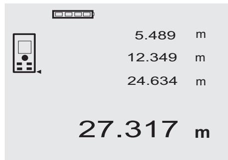
The tool can, of course, be switched on again at any time by pressing the “Measure” button. Pressing the C-button clears all currently displayed values.
