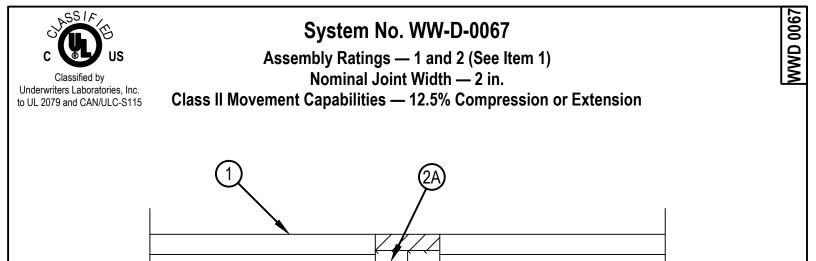
1. Wall Assembly — Nonbearing 1 or 2 hr fire rated gypsum board/steel stud assembly constructed of the materials and in the manner described in the individual U400 or V400 Series Wall or Partition Design in the UL Fire Resistance Directory and shall include the following construction features:
