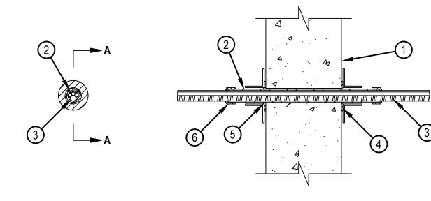
1. Wall Assembly — Min 6 in. (152 mm) thick reinforced lightweight or normal weight (100-150 pcf or 1600-2400 kg/m3) concrete Wall may also be constructed of any UL Classified Concrete Blocks\*. Max diam of opening is 1-1/2 in. (38 mm). See Concrete Blocks (CAZT) category in the Fire Resistance Directory for names of manufacturers.
