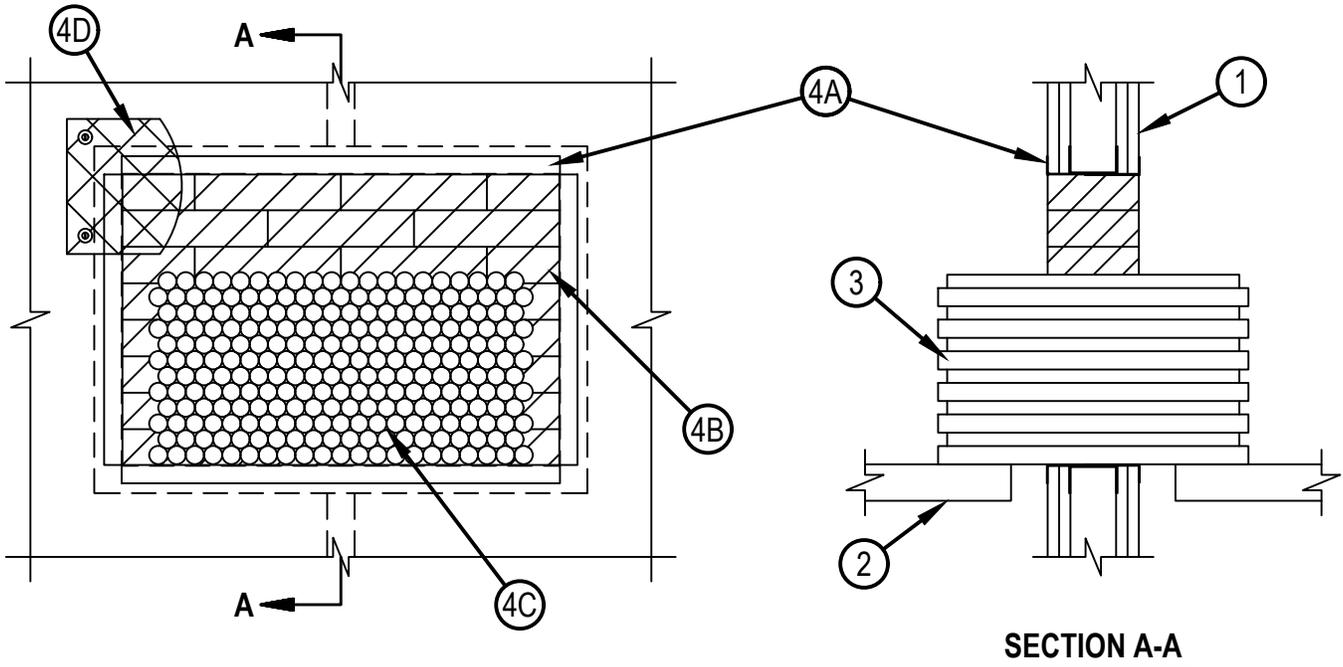
1. Wall Assembly — The 1 or 2 hr fire-rated gypsum board/stud wall assembly shall be constructed of the materials and in the manner specified if the individual U300, U400, V400 or W400 Series Wall and Partition Designs in the Fire Resistance Directory and shall include the following construction features:
