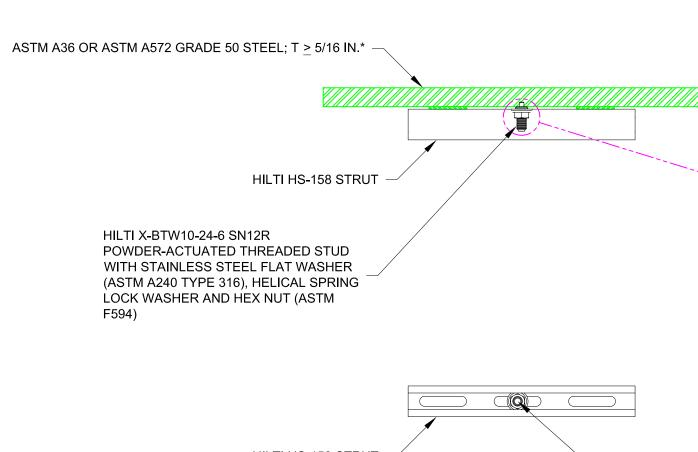
HILTI X-BTW10-24-6 SN12R POWDER-ACTUATED THREADED STUD WITH STAINLESS STEEL FLAT WASHER (ASTM A240 TYPE 316), HELICAL SPRING LOCK WASHER AND HEX NUT (ASTM F594)
