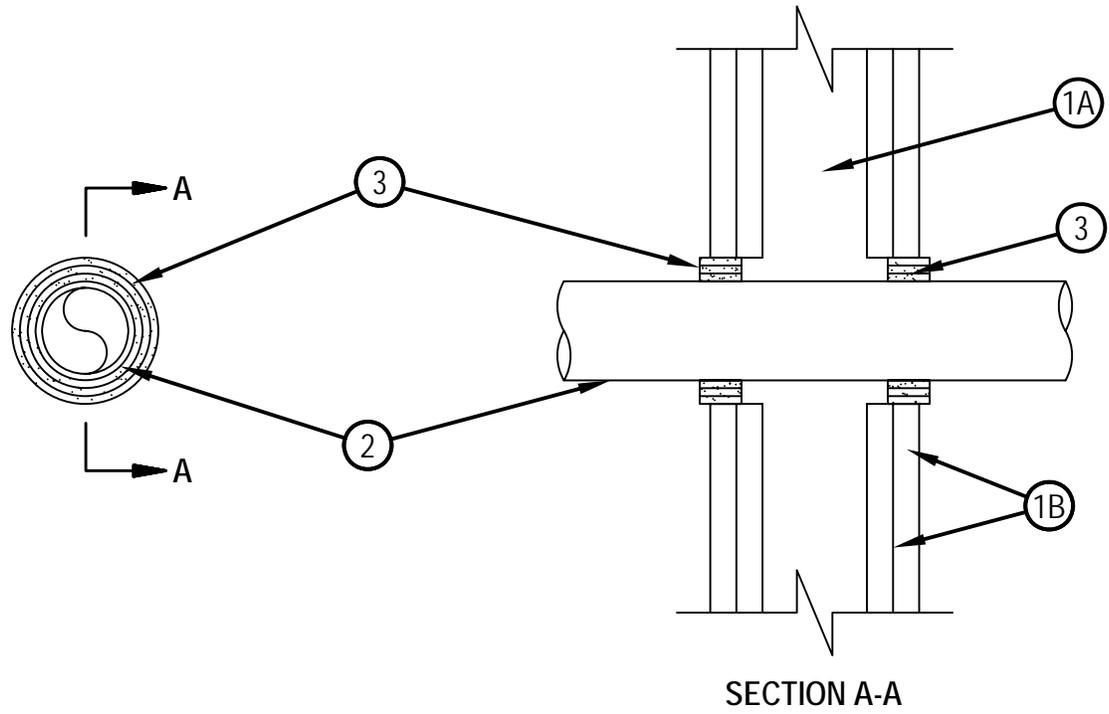
1. Wall Assembly -- The fire-rated gypsum wallboard/stud wall assembly shall be constructed of the materials and in the manner specified in the individual U300 or U400 Series Wall and Partition Designs in the UL Fire Resistance Directory and shall include the following construction features:
