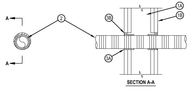
System tested with a pressure differential of 50 Pa between the exposed and the unexposed surfaces with the higher pressure on the exposed side.
