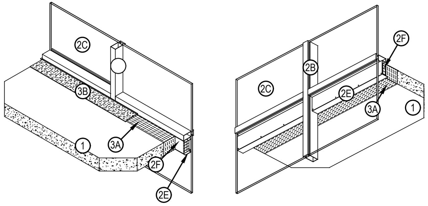
1. CONCRETE FLOOR ASSEMBLY : 2 hour rated concrete floor assembly made from either lightweight or normal weight concrete with a density of 100 to 150 pcf, having a min. thickness of 6 in. at the joint face. When a longitudinal recess (blockout) is required to contain an architectural joint system, increase concrete floor assembly thickness to maintain a min. thickness of 6 in. and accommodate depth of blockout formed in the concrete: blockout width unrestricted.
