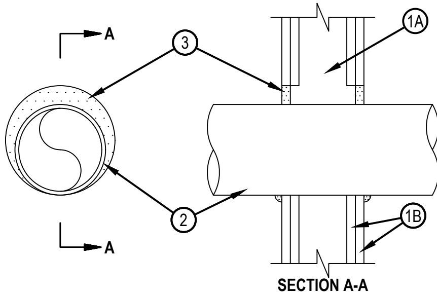
1. Wall Assembly — The 1 or 2 hr fire-rated gypsum wallboard/stud wall assembly shall be constructed of the materials and in the manner specified in the individual U300 or U400, U400, and V400 Series Wall and Partition Designs in the UL Fire Resistance Directory and shall include the following construction features:
