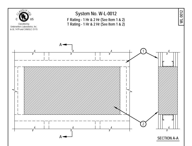
1. Wall Assembly -- The 1 or 2 hr fire-rated gypsum board/stud wall assembly shall be constructed of the materials and in the manner described in the individual U400 Series Wall or Partition Design in the UL Fire Resistance Directory and shall include the following construction features:
