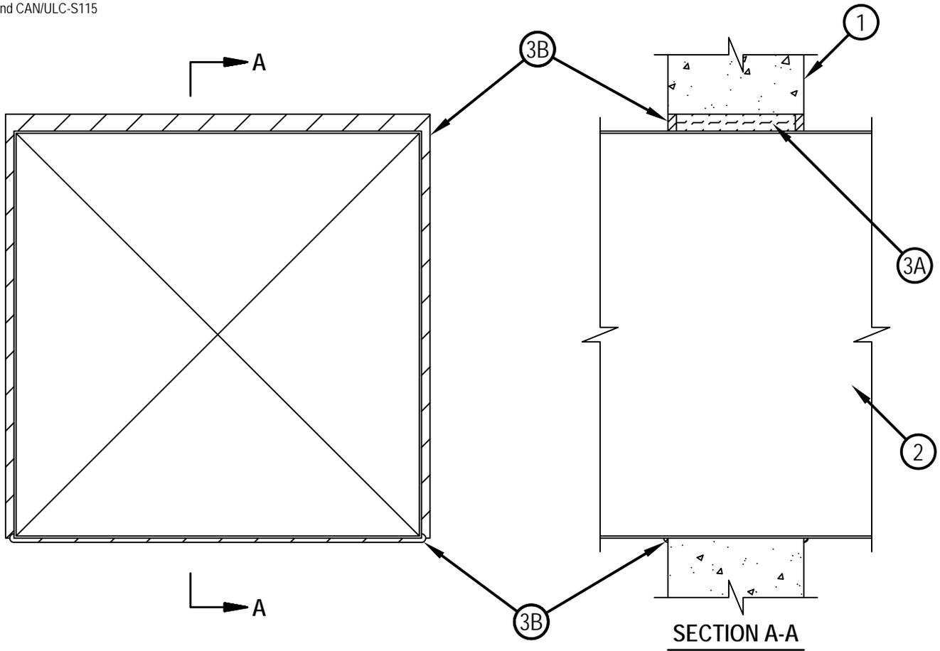
1. Wall Assembly — Min 6 in. (152 mm) thick reinforced lightweight or normal weight (100-150 pcf or 1600-2400 kg/m<sup>3</sup>) concrete. Wall may also be constructed of any UL Classified Concrete Blocks\*. Max size of opening is 625 sq in. (4032 cm<sup>2</sup>) with a max dimension of 25 in. (635 mm).
