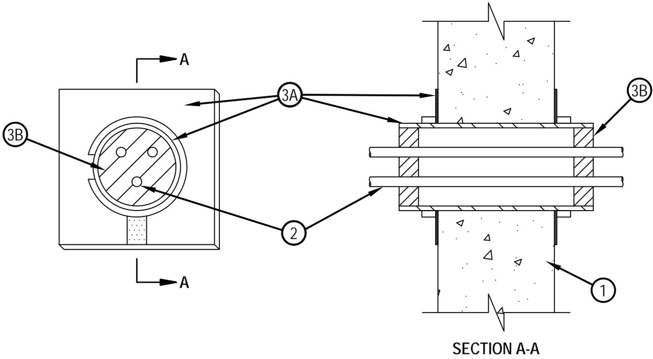
1. Wall Assembly — Min 6 in. (152 mm) thick reinforced lightweight or normal weight (100-150 pcf or 1600-2400 kg/m<sup>3</sup>) concrete. Wall may also be constructed of any UL Classified Concrete Blocks\*.
