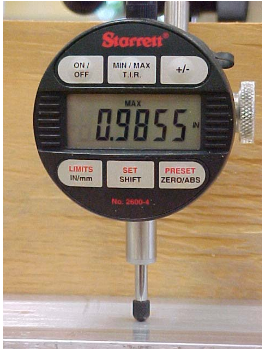
Photo No. 14 Beam Deflection Construct - Deflection Gauge Detail
