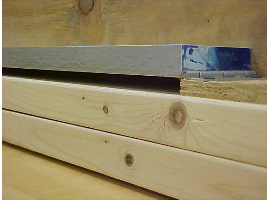
Photo No. 11 Beam Deflection Construct - 1/2" Cavity Detail
