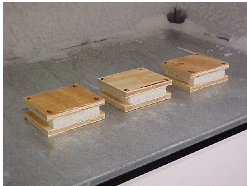
Photo No. 8 Dimensional Stability - Cold Conditioning
