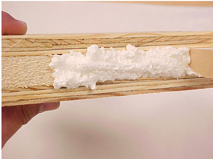
Photo No. 6 Dimensional Stability Construct - Filled
