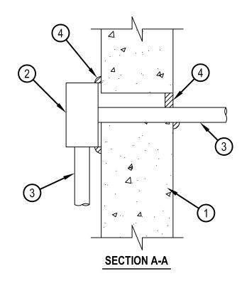
1. Wall Assembly — Min 5-5/8 in. (143 mm) reinforced lightweight or normal weight (100-150 pcf or 1600-2400 kg/m3) concrete. Wall may also be constructed of any UL Classified Concrete Blocks\*. Diam of opening to be min 1/2 in. (13 mm) larger than outside diam of through penetrant. Max diam of opening is 2-1/4 in. (57 mm).
