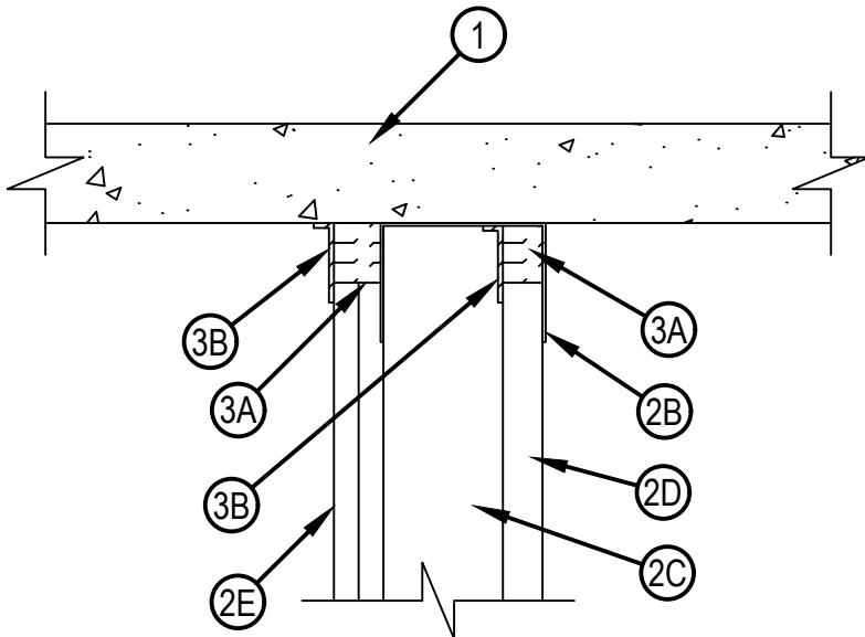
1. Floor Assembly — Min 2-1/2 in. (64 mm) thick lightweight or normal weight (100-150pcf or 1600-2400 kg/m<sup>3</sup>) structural concrete. Floor may also consist of any min 6 in. (152 mm) thick UL Classified hollow-core Precast Concrete Units\*.
