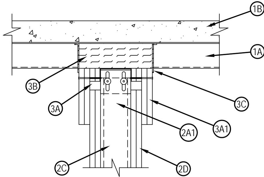
1. Floor Assembly — The fire-rated fluted steel deck/concrete floor assembly shall be constructed of the materials and in the manner described in the individual D700 or D900 Floor-Ceiling Design in the UL Fire Resistance Directory and shall include the following construction features:
