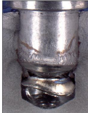
Clamping and welding effect of base material on the X-BT-MF shank
