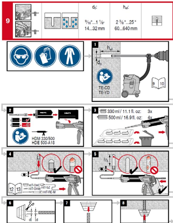
**Adhesive anchoring system for rebar and anchor fastenings in concrete**
