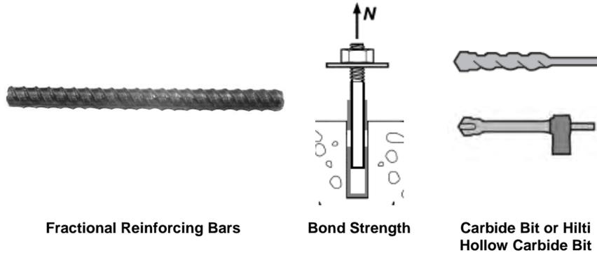
**TABLE 7—BOND STRENGTH DESIGN INFORMATION FOR FRACTIONAL REINFORCING BARS IN HOLES DRILLED WITH A HAMMER DRILL AND CARBIDE BIT (OR HILTI HOLLOW CARBIDE DRILL BIT)<sup>1,2,3,4</sup>**
