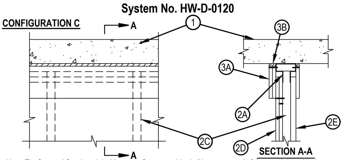
1. Floor Assembly — The fire-rated fluted steel deck/concrete floor assembly shall be constructed of the materials and in the manner described in the individual D900 Floor-Ceiling Design in the UL Fire Resistance Directory. The hourly fire rating of the floor assembly shall be equal to or greater than the hourly fire rating of the wall assembly. The floor assembly shall include the following construction features:
