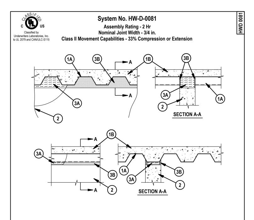
1. Floor Assembly — The fire-rated fluted steel floor unit/concrete floor assembly shall be constructed of the materials and in the manner described in the individual D700 or D900 Floor-Ceiling Design in the Fire Resistance Directory and shall include the following construction features:
