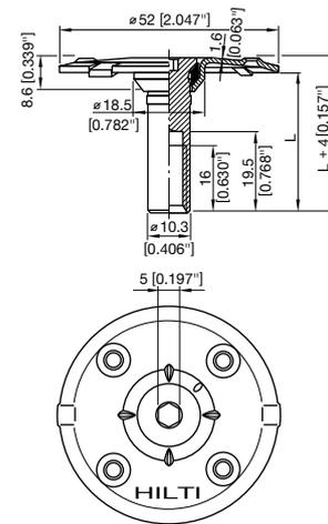
**Important:** The X-FCM-R system is not designed or intended to resist shear loads.
