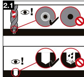
2.1 Pre-drill until shoulder grinds a shiny ring. The drill hole and the area around drilled hole must be clean and free from liquids and debris
