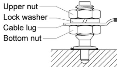
**Double point connection only for X-BT-ER M6/W6 and X-BT-ER M8**
