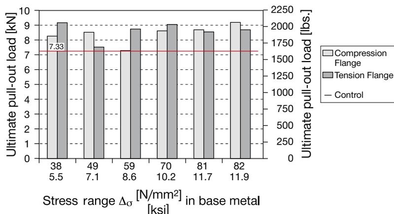
7.33 kN = Ultimate pull-out on the sample before stress was applied (control).
