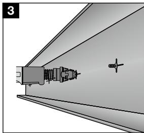
3 Drive fastener only with **DX 351 BT** tool and 6.8/M brown cartridge.
