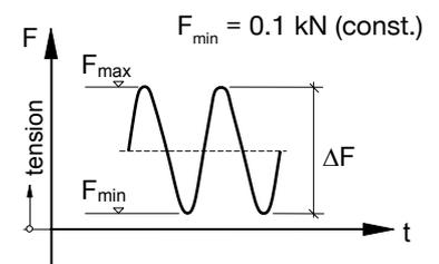
**Figure 4.** Principle sketch of cyclic tension tests
