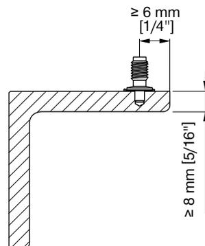
**3.3.4 Application limit/thickness of base material**
