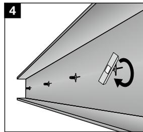
4 Screw on the connector and hand tighten. ( $T_{rec} \leq 8 \text{ Nm} / 5.9 \text{ ft-lb}$ )
