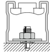
**Fastening MQ brackets and bases for raised floor**
