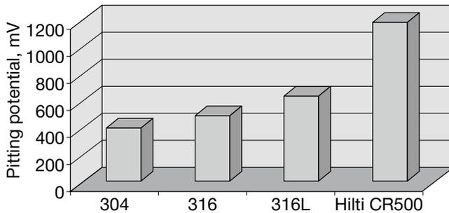
Potential-static test carried out with rods and nails in synthetic sea water as per ASTM D 1141
