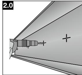
2.0 Pre-drill with **TX-BT 4/7** step shank drill bit.
