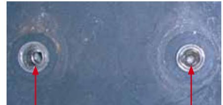
Drilled holes after 90 days salt spray test and after pull-out of the X-BT fasteners. These holes appear clean and no evidence of corrosion is visible.
