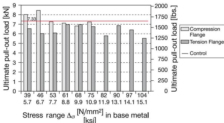
7.33 kN = Ultimate pull-out on the sample before stress was applied (control). No measurements taken on the compression flange in the high stress area due to position of the press.
