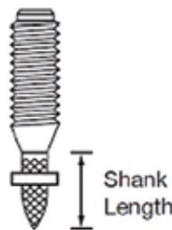
FIGURE 1—POINTED-TIP THREADED STUD
