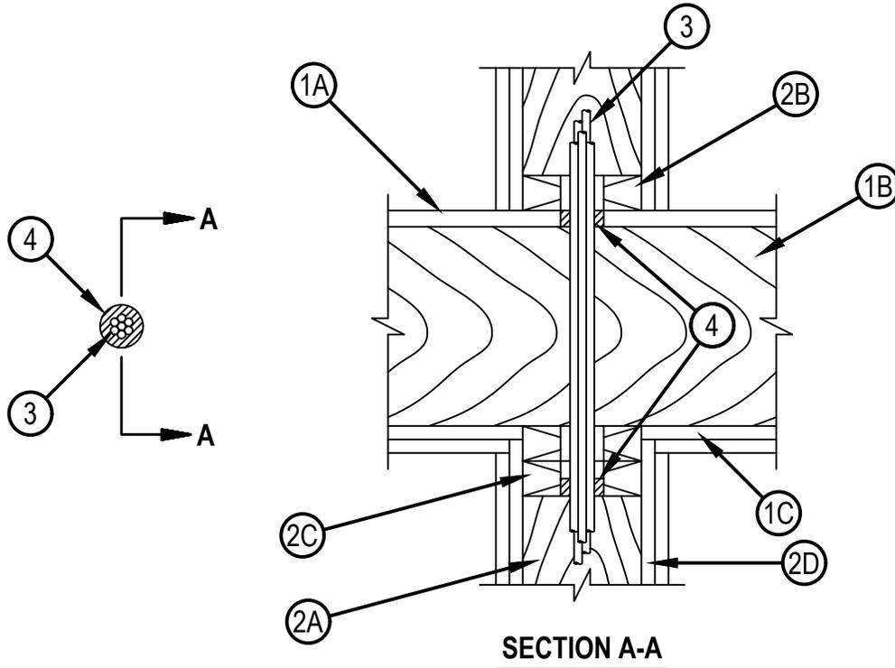
1. Floor-Ceiling Assembly — The 1 or 2 hr fire-rated solid or trussed lumber joist floor-ceiling assembly shall be constructed of the materials and in the manner specified in the individual L500 Series Floor-Ceiling Designs in the UL Fire Resistance Directory. The general construction features of the floor-ceiling assembly are summarized below:
