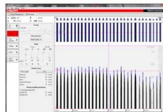
Quickscan data analysis of depth of concrete cover, displayed using the Hilti PROFIS Detection PC application.
