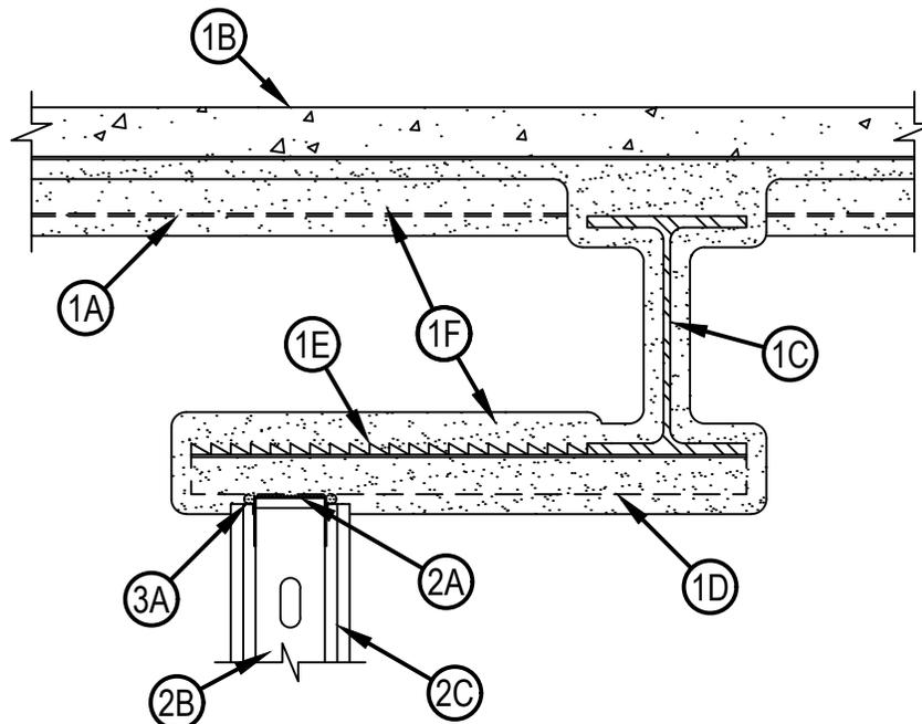
1. Floor Assembly — The fire-rated fluted steel deck/concrete floor assembly shall be constructed of the materials and in the manner described in the individual D700 or D900 Series Floor-Ceiling Design in the UL Fire Resistance Directory and as noted below. The hourly fire rating of the floor assembly shall be equal to or greater than the hourly fire rating of the wall assembly. The floor assembly shall include the following construction features:
