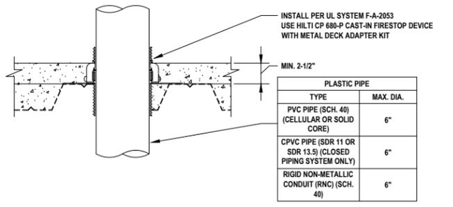
**3** PLASTIC PIPE THROUGH CONCRETE OVER METAL DECKING (2-HR.)
