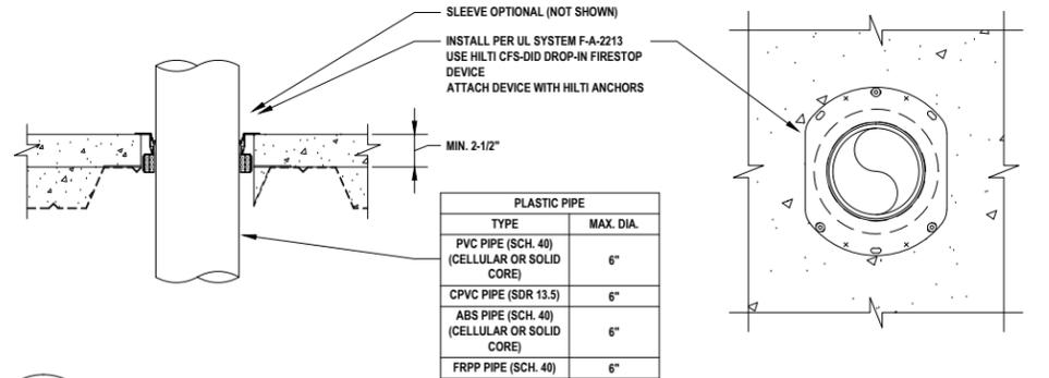
**6** PLASTIC PIPE THROUGH CONCRETE OVER METAL DECKING (2-HR.)
