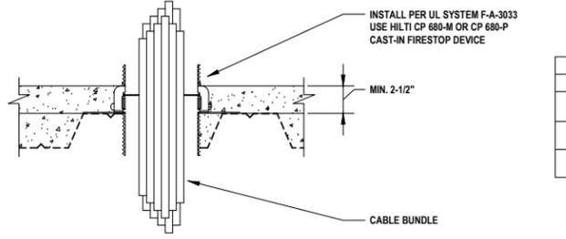
**5** CABLE BUNDLE THROUGH CONCRETE OVER METAL DECKING (2-HR.)
