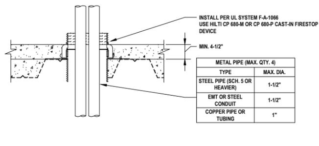
**2** MULTIPLE METAL PIPES THROUGH CONCRETE OVER METAL DECKING (2-HR.)
