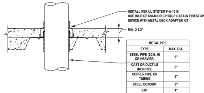
**1** METAL PIPE THROUGH CONCRETE OVER METAL DECKING (2-HR.)
