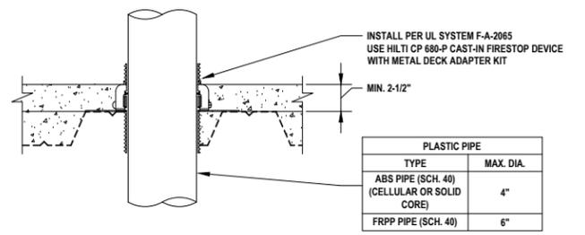
**4** PLASTIC PIPE THROUGH CONCRETE OVER METAL DECKING (2-HR.)
