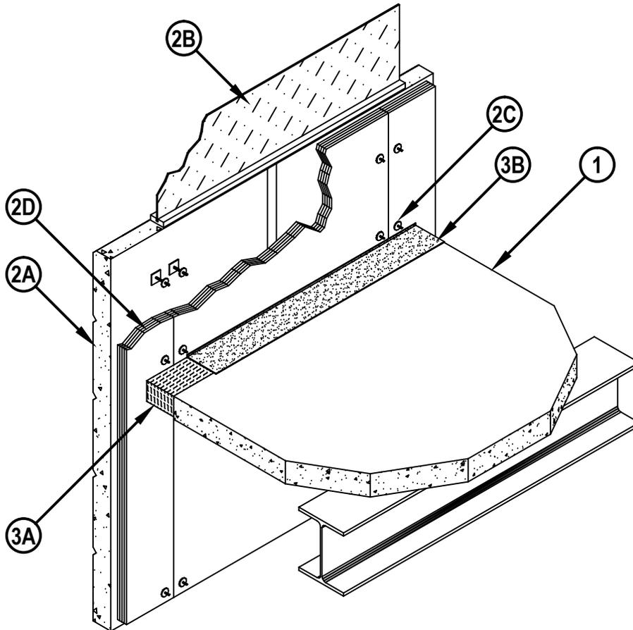
1. Floor Assembly — Min 4-1/2 in. (114 mm) thick steel-reinforced lightweight or normal weight (100-150 pcf or 1600-2400 kg/m<sup>3</sup>) structural concrete. Floor assembly to be supported at perimeter edges by spandrel beams having a Restrained or Unrestrained Beam Rating of 2 hr. Edge of concrete floor to be max 8 in. from interior surface of spandrel panel (Item 2A).
