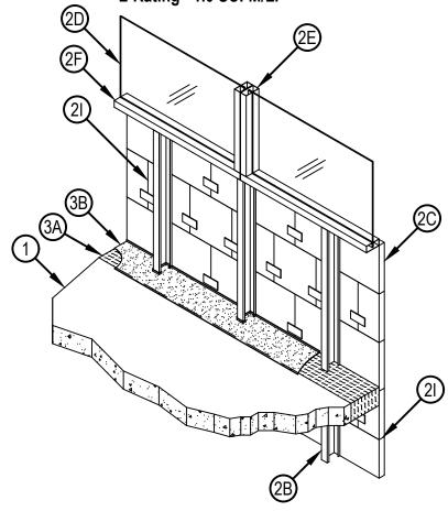
1. CONCRETE FLOOR ASSEMBLY: Two hour rated concrete floor assembly made from either lightweight or normal weight concrete with a density of 100-150 pcf, with a min. thickness of 4-1/2 in. at the joint face. Overall slab thickness may vary to accommodate various blockout depths (longitudinal recesses) formed in the concrete, to house the architectural cover plate. The blockout width may also vary without restriction.
