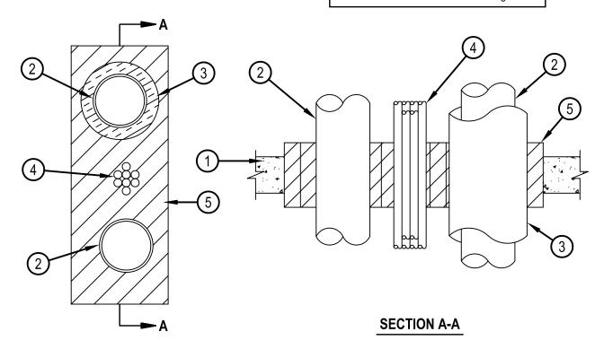
1. Floor, Roof or Wall Assembly — The fire-rated floor- or roof-ceiling assembly shall be constructed of Precast Autoclaved Aerated Concrete\* in the manner specified in Design Nos. K908 or P931, respectively, and the fire rated wall assembly shall be constructed of Precast Autoclaved Aerated Concrete\* in the manner specified in Design Nos. U916 or U917 in the UL Fire Resistance Directory. Max area of opening is 384 sq in. (2477 cm²) with max dimension of 32 in. (813 mm).
