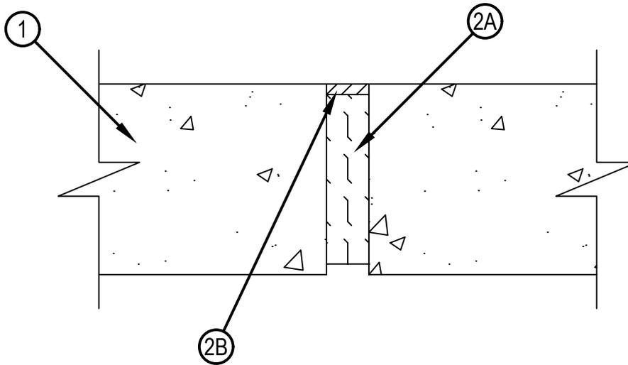
1. Floor Assembly — Min 4-1/2 in. (114 mm) thick reinforced lightweight or normal weight (100-150 pcf 1600-2400 kg/cu meter) concrete.
