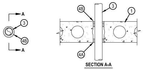
1. Floor or Wall Assembly — See Configuration A above. Reinforced lightweight or normal weight (100-150 pcf or 1600-2400 kg/cu meter) concrete as specified in the Table in Item 4 below. Wall may also be constructed of any UL Classified Concrete Blocks\*. Max diam of sleeved opening is 32 in. (813 mm).
