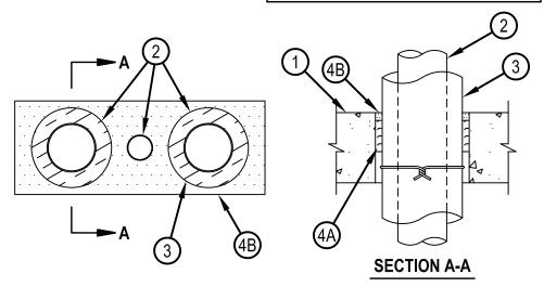
1. Floor or Wall Assembly — Min 4-1/2 in. (114 mm) thick reinforced lightweight or normal weight (100-150 pcf or 1600-2400 kg/m3) concrete. Wall may also be constructed of any UL Classified Concrete Blocks\*. Max area of opening is 96 sq in. (619 cm2) with max dimension of 16 in. (406 mm).
