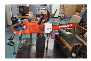
Weight and measures for this modified lab equipment were based on ASTM F1414 Test Methods for cut resistance testing of Chainsaw Leg Protective Devices { Note this ASTM F1414 Reference was only the guide used to mount the Hilti Battery Saw and this lab set up is not considered as an actual ASTM F 1414 testing device , this set up is only to simulate the parameters as close as possible to gather data specific to the power head shown above}
