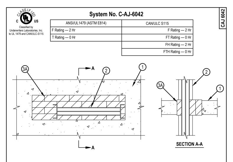
1. Floor or Wall Assembly — Min 4-1/2 in. (114 mm) thick reinforced lightweight or normal weight (100-150 pcf or 1600-2400 kg/m3) concrete floor or wall. Wall may also be constructed of any UL Listed Concrete Blocks\*. Max area of opening is 240 in.2 (1548 mm2) with max dimension of 30 in. (762 mm).
