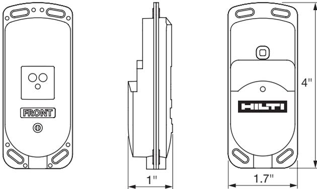
Hilti embedded wireless sensors continuously capture, store and send data via cellular system with the Hilti Gateway to our Hilti Cloud software for monitoring the strength and temperature of the in-field concrete. You can then view the data through our Hilti mobile app or on a browser.
