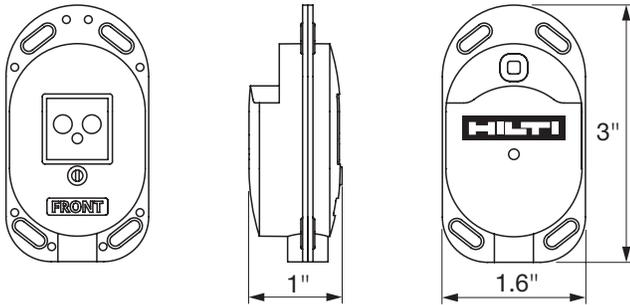
Hilti embedded wireless sensors continuously capture, store and send data via Bluetooth® to our Hilti cloud software for monitoring the strength and temperature of the in-field concrete. You can then view the data through our Hilti mobile app or through a browser.
