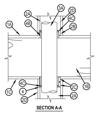
System tested with a pressure differential of 2.5 Pa between the exposed and the unexposed surfaces with the higher pressure on the exposed side.
