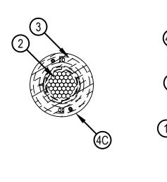
1. Floor or Wall Assembly — Reinforced lightweight or normal weight (100-150 pcf or 1600-2400 kg/m3) concrete. Min 4-1/2 in. (114 mm) thick floors and min 5 in. (127mm) thick walls. Wall may also be constructed of any UL Classified Concrete Blocks\*. Floor may also be constructed of any min 6 in. thick UL Classified hollow-core Precast Concrete Units\*. Opening in floor or wall to be max 3 in. (76 mm) diam for 2 in. (51 mm) device and max 5 in. (127 mm) diam for 4 in. (102 mm) device.
