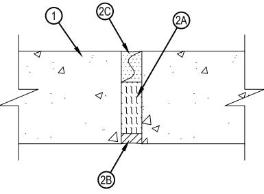
1. Wall Assembly —Min 4-1/2 in. (112 mm) thick reinforced lightweight or normal weight (100-150 pcf or 1600-2400 kg/m3) structural concrete. Wall may also be constructed of any UL Classified Concrete Blocks \*.
