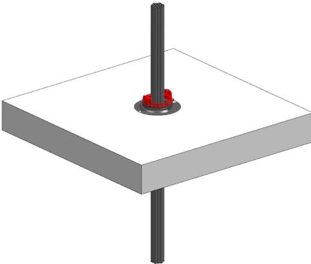
Cables to be tightly bundled within the device and rigidly supported on both sides of floor or wall assembly.
