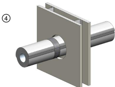
The radial seams are butted end to end without overlap. Apply 3 in. wide aluminum foil tape or FSK tape over the radial seam and overlap 2 in. onto it.
