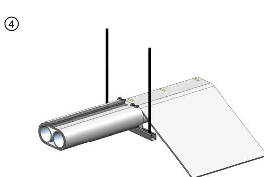
Install adjacent Layer 1 wrapped section as per previous instructions for aligned seam with sealant only.
