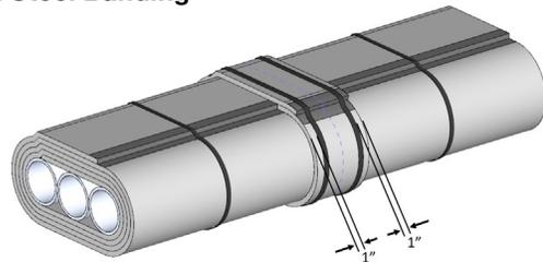
Secure collar with 1/2 in wide stainless-steel banding located 1 in. from each edge of collar as shown on the picture.
