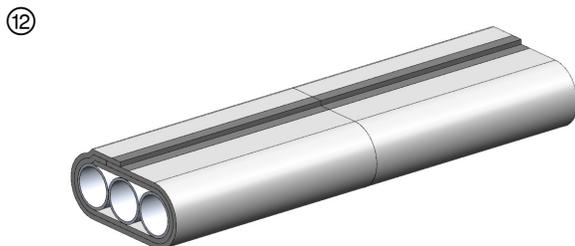
Secure Layer 2 with 3 in. wide aluminum foil tape or FSK tape covering the full length of the longitudinal seam
