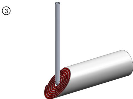
Apply 1/8 in. depth of Hilti CP 606 or FS-ONE MAX to be applied to cover 45 degree cut edge on one section.
