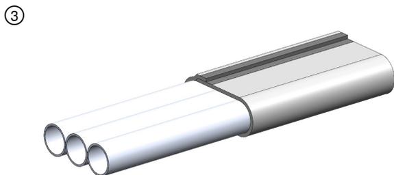
Wrap Hilti Endo-Shield tightly around the tubing overlapping 2 in. at the longitudinal seam. Apply 3 in. wide aluminum foil tape or FSK tape centered for the full length of the longitudinal seam.
