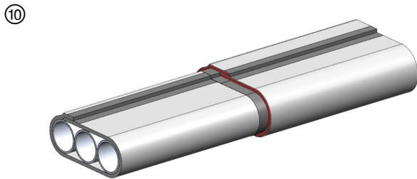
Prior to installing the adjacent wrapped section, apply 1/8 in. wet thickness of Hilti CP 606 or FS ONE MAX over the entire edge of Hilti Endo-Shield Layer 2.
