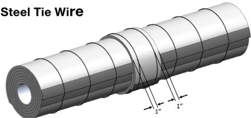
Secure final wrap with min 18 GA steel tie wire located 1in from each collar edge of collar.
