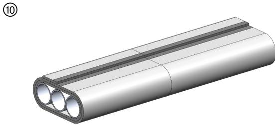
Apply 3 in. wide aluminum foil tape or FSK tape over the longitudinal seam.
