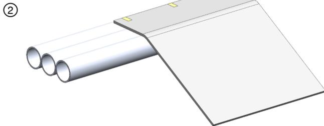
Layer 1: Tape Endo-Shield to the pipe with min 1/2 in. wide filament tape, FSK tape or aluminum foil tape.
