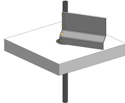
One layer of pipe covering shall be continuously wrapped around the device sleeve and penetrant.
