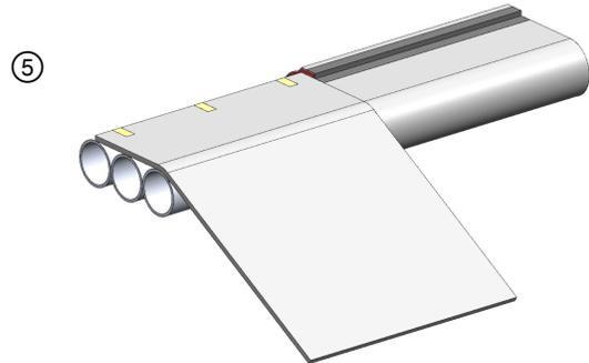
Wrap adjacent section continuously per previous instructions. Additional wrapped sections are added to insulate all straight runs of tubing.
