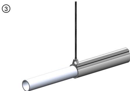
Wrap Hilti Endo-Shield tightly around the tubing overlapping 2 in. at the longitudinal seam. Apply 3 in. wide aluminum foil tape or FSK tape over the longitudinal seam.
