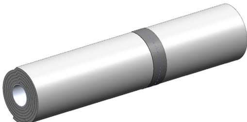
Layer 3, 4, 5: As required wrap third, fourth or fifth layer of Hilti Endo-Shield in the same manner as Layer 2 maintaining min 2 in. overlap of radial seams at each layer, to obtain desired rating.
