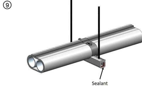
Apply 1/8 in. thick bead of Hilti CP 606 or FS-ONE MAX to the inner surface of the strut ends.
