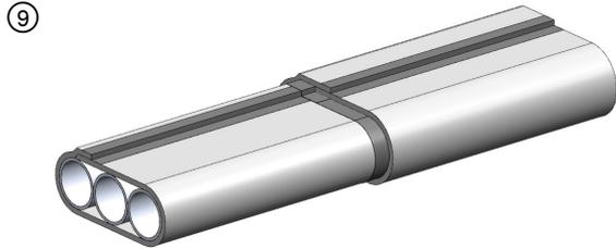
Tightly wrap Layer 2 over Layer 1 and overlap the longitudinal seam by 2 in. Cover the full length of the longitudinal with 3 in. wide aluminum foil tape or FSK tape.
