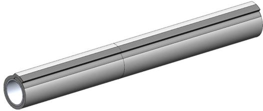
Apply 3 in. wide aluminum foil tape or FSK tape centered for the full length of the longitudinal seam.
