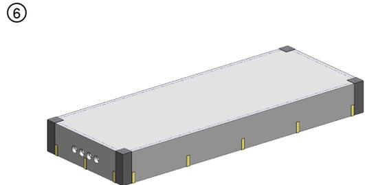
Seal corners with aluminum foil or FSK tape.
