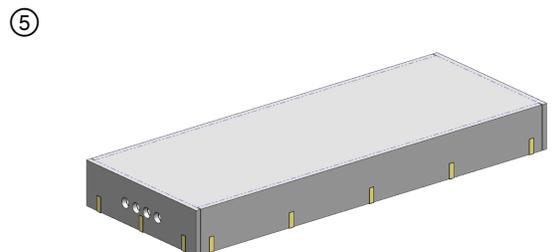
At the corners of the box, wrap material is trimmed at top and bottom so that it is flush with the wrap on the sides.
