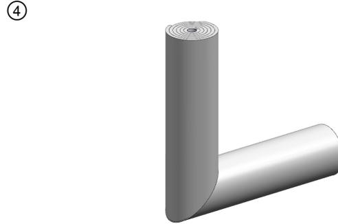
Install the adjacent continuously wrapped section. Both sections of Hilti Endo-Shield shall be slid together while aligning the 45 degree angled cuts.
