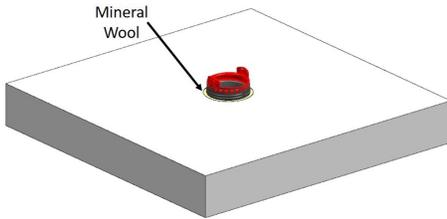
Min 4 in. (102 mm) thickness of min 4 pcf. (64 kg/m<sup>3</sup>) mineral wool batt insulation firmly packed into annular space between firestop device and opening as a permanent form. Packing material to be installed flush with bottom of floor and recessed from top surface of floor or from both surfaces of wall to accommodate the required thickness of fill material.
