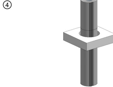
Install the adjacent continuously wrapped section. A 2 in. overlap of longitudinal seam shall be included for each layer required.
