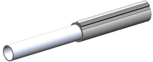
Wrap Hilti Endo-Shield tightly around the conduit overlapping 2 in. at the longitudinal seam. Apply 3 in. wide aluminum foil tape or FSK tape centered for the full length of the longitudinal seam.
