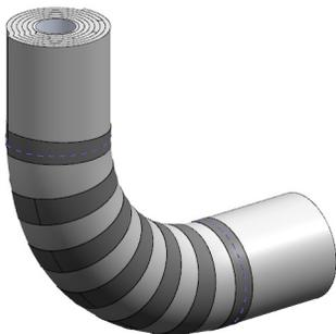
As per listing HI/AF 120-01. The elbow longitudinal seam of Layer 2 is located at the short radius of the elbow. The elbow longitudinal seam of Layer 3 is located at the middle radius of the elbow, rotated 90 degrees from the longitudinal seam of Layer 2. The elbow longitudinal seam for Layer 4 is located at the middle radius of the elbow, rotated 180 degrees from the longitudinal seal of Layer 3. The elbow longitudinal seam for Layer 5 (if necessary) is located at the long radius of the elbow.
