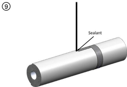
LAYER 3,4,5: As required wrap third, fourth or fifth layer of Hilti Endo-Shield in the same manner as Layer 2 to obtain desired rating. Apply 1/8 in. wet thickness of Hilti CP 606 or FS-ONE MAX to threaded rod penetration and each layer relief cuts.
