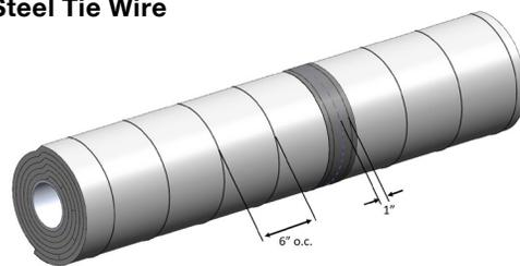
The outer layer is secured with min 18 GA steel tie wire located 1 in. from each radial seam. Space the steel tie wire 6 in. on center between the seam.
