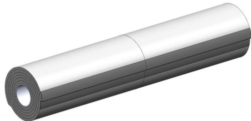
Hilti Endo-Shield may be continuously wrapped around the conduit. Using min 1/2 in. wide filament tape, FSK tape or aluminum foil tape, attach leading edge of Hilti Endo-Shield onto the conduit and wrap continuously.
