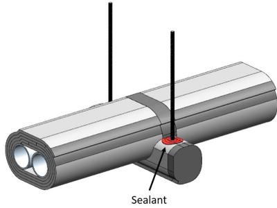
Apply 1/8 in. thick bead of Hilti CP 606 or FS-ONE MAX to outer diameter of the threaded rod penetration.
