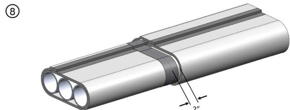
Offset the Layer 2 radial seam 2 in. from the radial seam of Layer 1. Tightly wrap Layer 2 over Layer 1 and overlap the longitudinal seam by 2 in. Cover the full length of the longitudinal and radial seam with 3 in. aluminum foil tape or FSK tape.
