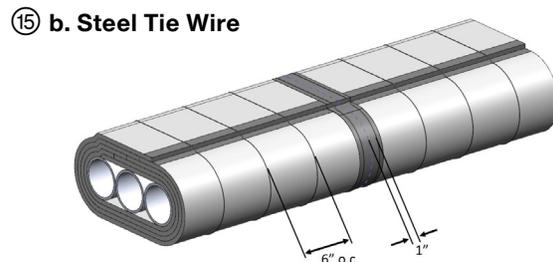
Secure outer layer with min 18 GA steel tie wire located 1 in. from each radial seam. Space the steel tie wire 6 in. on center between the seam.
