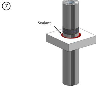
Min 1/2 in. (13 mm) thickness of Hilti FS-ONE MAX applied within the annulus, flush with top surface of floor or with both surfaces of wall.
