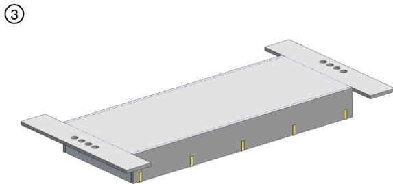
At corners of steel box, wrap cut horizontally or vertically, extending from corner of steel box to edge of wrap material.
