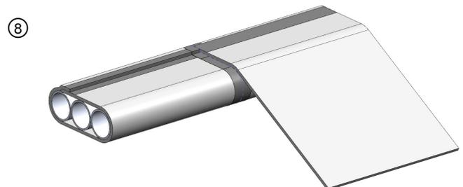
Layer 2: Wrap second layer of Hilti Endo-Shield in the same manner as Layer 1. The start of Layer 2 begins at the longitudinal seam of Layer 1, secured with 3 in. wide aluminum foil tape or FSK tape covering the full length of the seam.
