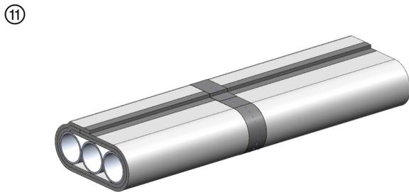
The radial seams are butted end to end without overlap. Apply 3 in. wide aluminum foil tape or FSK tape over the radial seam and overlap 2 in. onto itself.
