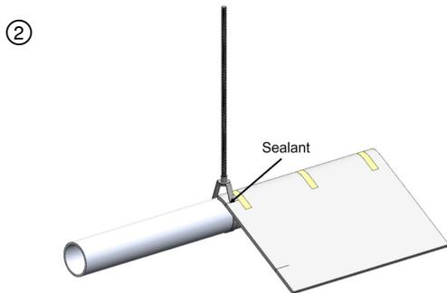
Apply relief cuts positioned to contour around the loop hanger. Attach Layer 1 using min 1/2 in. wide filament tape, FSK tape or aluminum foil tape. Apply 1/8 in. bead wet thickness of Hilti CP 606 or FS-ONE MAX to the relief cuts.
