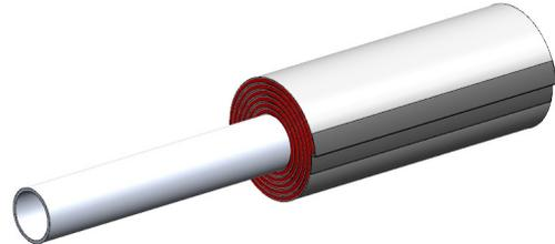
Prior to installing the adjacent continuously wrapped section, apply 1/8 in. wet thickness of Hilti CP 606 or FS-ONE MAX over the entire edge of Hilti Endo-Shield.
