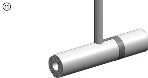
Wrap two layers of Hilti Endo-Shield around the threaded rod continuously adding 4 in. overlap to the final layer or with individual layers each one with a 2 in. overlap. Apply 3 in. wide aluminum foil tape or FSK tape over the longitudinal seam. *The threaded rod needs to be wrapped to the concrete interface.*
