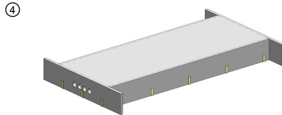
Wrap material folded to maintain contact with back and four sides of steel box.
