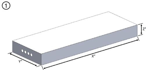
Max 14-3/8 in. (365 mm) wide by 39 in. (991 mm) by max 3-7/8 in. (98 mm) by minimum 20 gauge steel electrical panel box, steel utility box, or steel med-gas valve box with hinged steel door and mounting flange.
