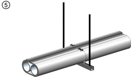
Apply 3 in. wide aluminum foil tape or FSK tape over the longitudinal seam.
