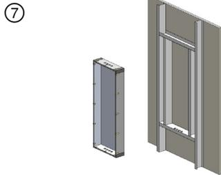
Wall framing may consist of steel channel studs. Steel studs to be min 3-5/8 in. (92 mm) wide and spaced max 24 in. (610 mm) OC. Additional studs installed horizontally at the top and bottom of the steel box. Additional studs installed vertically as required for steel box attachment.
