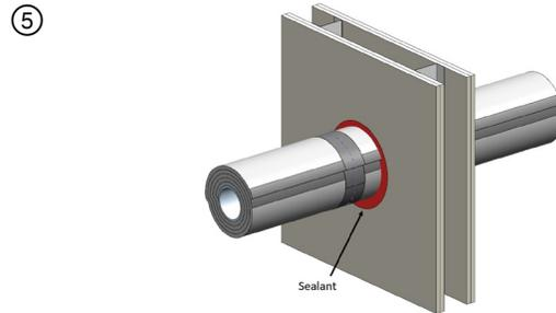
Min 5/8 in. (16 mm) thickness Hilti FS-ONE MAX applied within the annulus, flush with both surfaces of wall. At the point contact location between pipe covering and gypsum board, a min 1/2 in. (13 mm) diam bead of fill material shall be applied at the pipe covering/gypsum board interface on both surfaces of wall.
