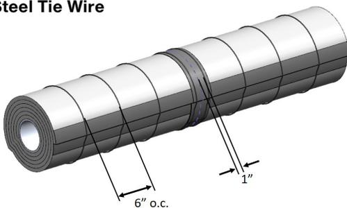
The outer layer is secured with min 18 GA steel tie wire located 1 in. from each radial seam. Space the steel tie wire 6 in. on center between the seam.
