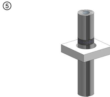
The radial seams are butted end to end without overlap. Apply 3 in. wide aluminum foil tape or FSK tape over the seam and overlap.
