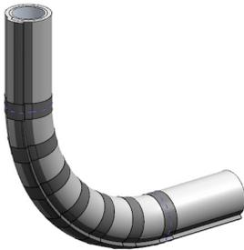
Apply 3 in. wide aluminum foil tape or FSK tape over the radial seams and overlap 2 in. back onto itself.
