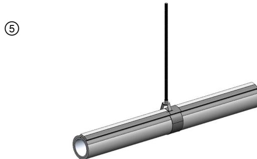
Apply 3 in. wide aluminum foil tape or FSK tape over the radial seam and overlap 2 in. onto itself. Add a piece of aluminum foil tape or FSK tape over relief cut.
