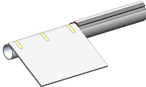
Wrap adjacent section per previous instructions. Additional wrap sections are added to insulate all straight runs of tubing.
