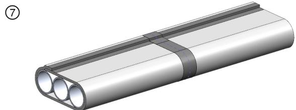
The radial seams are butted end to end without overlap. Apply 3 in. wide aluminum foil tape or FSK tape over the seam and overlap 2 in. onto itself.
