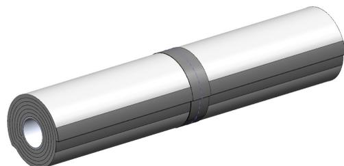
Wrap Hilti Endo-Shield continuously adding the number of layers required by the 3rd party tested firestop system. Apply 3 in. wide aluminum foil tape or FSK tape over the longitudinal seam. A 2 in. overlap of longitudinal seam shall be included for each layer required. For example, 4-layer system requires an 8 in. overlap on a final layer.
