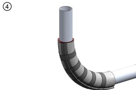
Prior to installing the adjacent straight sections, apply 1/8 in. wet thickness of CP 606 or FS One max over the entire edge of Hilti Endo-Shield Layer 1 (unless using collar protection).
