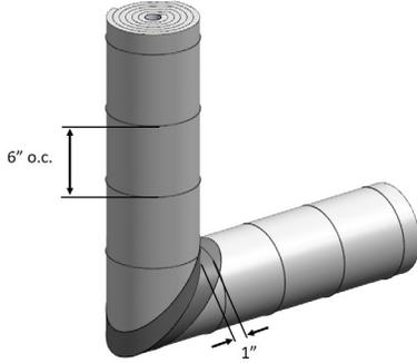
Secure elbow treatment with min. 18 Ga steel tie wire located 1" from interior radius of elbow treatment on both sections of Hilti Endo-Shield. Space the steel tie wire 6 in. on center.
