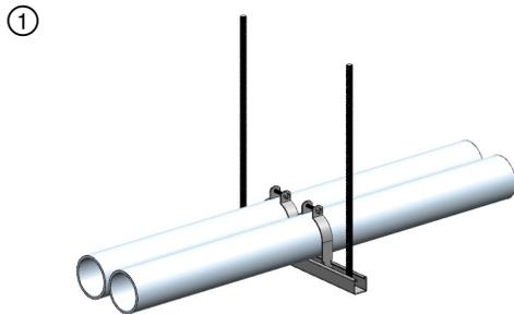
Traditionally a bank of critical conduits is supported by a strut assembly as shown on the drawing.
