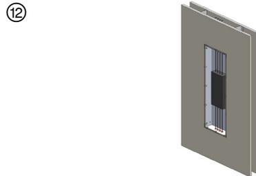
Min 1/2 in. (13 mm) thickness Hilti FS-ONE MAX or CP 618 Firestop Putty applied into ends of pipes, tubes or conduits that terminate inside box.
