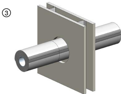
Install the adjacent continuously wrapped section. A 2 in. overlap of longitudinal seam shall be included for each layer required. Apply 3 in. wide aluminum foil tape or FSK tape over the longitudinal seam.
