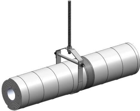
When HILTI Endo-Shield is wrapped prior to hanging with a loop hanger which fits the outer diameter of the HILTI Endo-Shield, there is no need to protect the support member for circuit integrity purposes.
