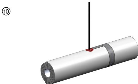
Apply 1/8 in. wet thickness Hilti CP 606 or FS-ONE MAX to outer diameter of the threaded rod penetration.
