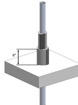
For a 2 hr. T, FT and FTH Rating, an additional layer of pipe covering shall be tightly wrapped around the first layer and extend min 6 in. (152 mm) above floor. All seams to overlap min 2 in. (51 mm) and to be sealed with FSK or foil tape.
