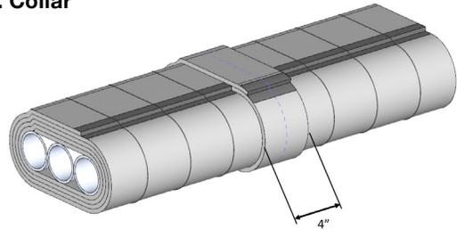
At radial seams and seams between the gore end segment and adjoining straight section, add an additional 4 in. wide section of Hilti Endo-Shield. Center over the radial seam of the final layer overlapping 2 in. at the longitudinal seam. Apply 3 in. wide aluminum foil tape or FSK tape over the longitudinal seam of the 4 in. wide section of Hilti Endo-Shield. Secure with Steel tie wire per 9b.
