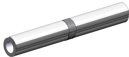
The radial seams are butted end to end without overlap. Apply 3 in. wide aluminum foil tape or FSK tape over the seam and overlap 2 in. back onto itself.
