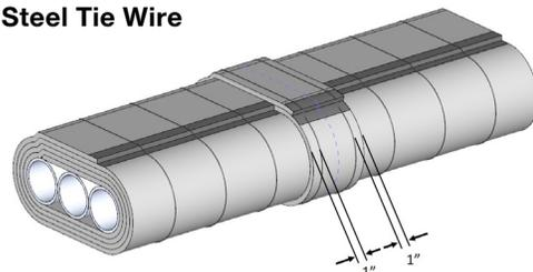
Secure collar with min 18 GA steel tie wire located 1 in. from each edge of collar.
