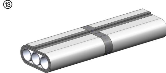
The radial seams are butted end to end without overlap. Apply 3 in. wide aluminum foil tape or FSK tape over the radial seam and overlap 2 in. back onto itself.
