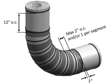
At the elbow, space the steel banding 2 in. on center at both at the short interior radius.
