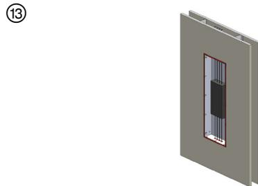
Min 1/4 in. (6 mm) bead of Hilti CP606 or FS-ONE MAX applied over exposed edge of CFP-ES Endo Shield prior to installing mounting flange of steel box.
