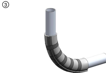
Apply 3 in. wide aluminum foil tape or FSK tape over the radial seams and overlap 2 in. back onto itself.
