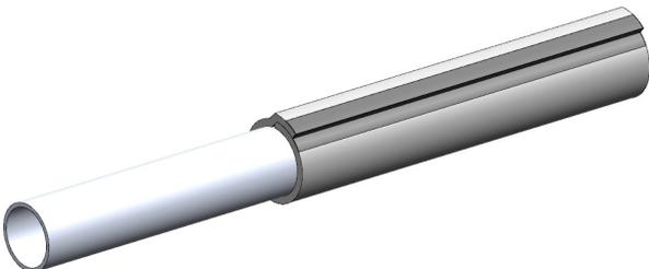
Wrap Hilti Endo-Shield tightly around the tubing overlapping 2 in. at the longitudinal seam. Apply 3 in. wide aluminum foil tape or FSK tape centered for the full length of the longitudinal seam.
