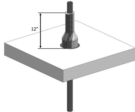
Extend layer min 12 in. (305 mm) above the floor, with a min 2 in. (51 mm) overlap at the seam. All seams to be sealed with FSK or foil tape. In walls, pipe covering to be installed on both sides of wall.
