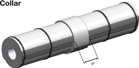
At radial seams and seams between the gore end segment and adjoining straight section, add an additional 4 in. wide section of Hilti Endo-Shield. Center collar over the radial seam of the final layer overlapping 2 in. at the longitudinal seam. Apply 3 in. wide aluminum foil tape or FSK tape over the longitudinal seam of the 4 in. wide section of Hilti Endo-Shield. Secure with steel banding per 9a.
