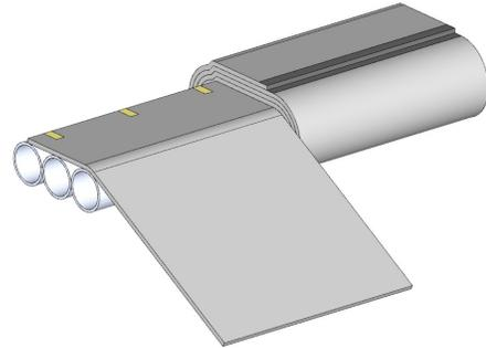
Wrap adjacent section continuously per previous instructions. Additional wrapped sections are added to insulate all straight runs of tubing.
