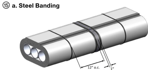
Secure outer layer with 1/2 in. wide stainless-steel banding located 1 in. from each radial seam. Space the steel banding 12 in. on center between seams.
