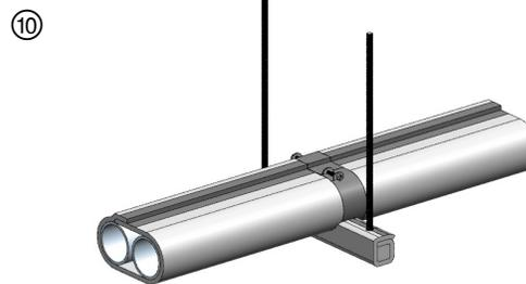
Cut a Hilti Endo-Shield plug to seal strut ends.
