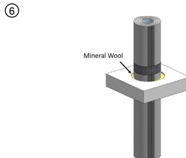
Min 4 in. (102 mm) thickness of min 4 pcf (64 kg/m<sup>3</sup>) mineral wool batt insulation compressed and firmly packed within annular space. Packing material to be recessed from top surface of floor or from both surfaces of wall to accommodate the required thickness of fill material.
