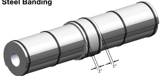
Secure section with 1/2 in wide stainless-steel banding located 1 in. from each edge of collar.
