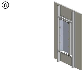
Sides of steel box attached from inside the box to wall framing using steel screws after application of wrap material.
