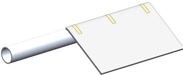
Layer 1: Tape Hilti Endo-Shield to the pipe with min 1/2 in. wide filament tape, FSK tape or aluminum tape.
