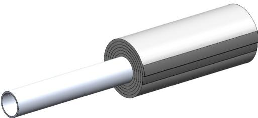
Wrap Hilti Endo-Shield continuously with the number of layers required by the 3rd party tested firestop system. A 2 in. overlap shall be included for each layer required. For example, 4-layer system requires an 8 in. overlap on a final layer. Apply 3 in. wide aluminum foil tape or FSK tape over the full length of the longitudinal seam.
