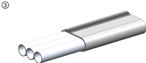
Wrap Hilti Endo-Shield tightly around the conduit bank overlapping 2 in. at the longitudinal seam. Apply 3 in. wide aluminum foil tape or FSK tape centered for the full length of the longitudinal seam.
