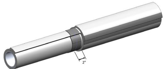
Wrap second layer of Hilti Endo-Shield in the same manner as Layer 1. Offset the Layer 2 radial seam 2 in. from the radial seam Layer 1. Tightly wrap Layer 2 over Layer 1 and overlap the longitudinal seam by 2 in. Cover the full length of the longitudinal and radial seam with 3 in. wide aluminum foil tape or FSK tape.
