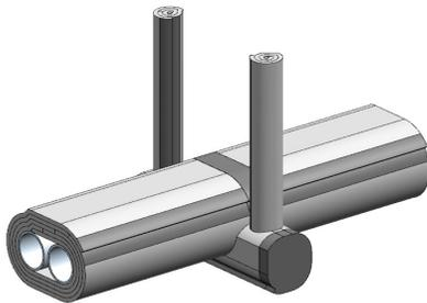
Wrap two layers of Hilti Endo-Shield around the threaded rod continuously adding 4 in. overlap to the final layer or with individual layers each one with a 2 in. overlap. Apply 3 in. wide aluminum foil tape or FSK tape over the longitudinal seam. *The threaded rod needs to be wrapped to the concrete interface.*
