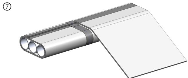
Layer 2: Wrap second layer of Hilti Endo-Shield in the same manner as Layer 1. The start of Layer 2 begins at the longitudinal seam of Layer 1, secured with 3 in. wide aluminum foil tape or FSK tape covering the full length of the seam.
