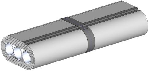
The radial seams are butted end to end without overlap. Apply 3 in. wide aluminum foil tape or FSK tape over the seam and overlap 2 in. onto itself.
