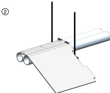
Add relief cuts and notches positioned to contour around the strut assembly. Attach Layer 1 using min 1/2 in. wide filament tape, FSK tape or aluminum foil tape.
