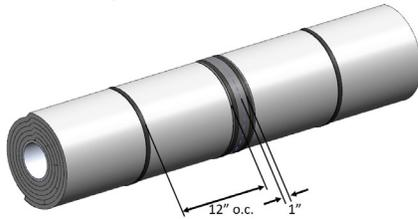
The outer layer is secured with 1/2 in. wide stainless-steel banding located 1 in. from each radial seam. Space the steel banding 12 in. on center.
