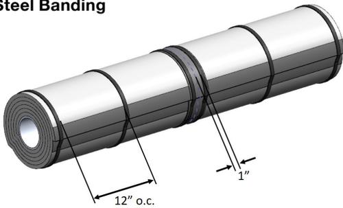
The outer layer is secured with 1/2 in. wide stainless-steel banding located 1 in. from each radial seam. Space the steel banding 12 in. on center.
