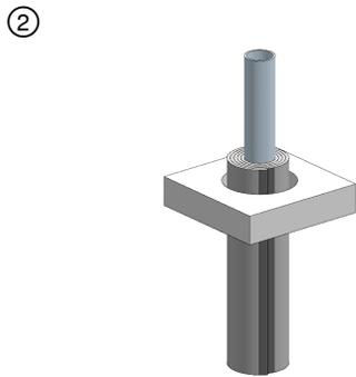
Wrap conduit per methods previously described to achieve desired rating. The annular space between pipe covering material and opening shall be min 1/2 in. (13 mm) to max 1-1/4 in. (32 mm).
