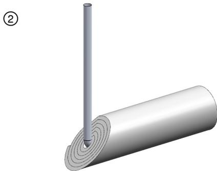
Each section to be cut to provide a 45 degree surface on the side of Hilti Endo-Shield closest to the elbow. Wrap Hilti Endo-Shield continuously adding the number of layers required by the 3rd party tested firestop system.
