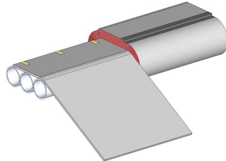
Hilti Endo-Shield may be continuously wrapped around the conduit bank. Using min 1/2 in. wide filament tape, FSK tape or aluminum foil tape, attach leading edge of Hilti Endo-Shield onto the conduit and wrap continuously.
