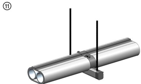
Apply 3 in. wide aluminum foil tape or FSK tape to wrap the strut ends.
