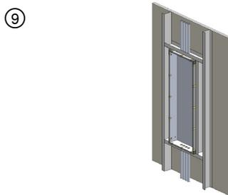
Top, bottom and/or sides of steel box may be penetrated by maximum twenty (20) total penetrants of nom 1/2 in. (13 mm) to 2 in. (51 mm) diam steel pipe, iron pipe, copper pipe or tube, steel conduit, EMT or flexible steel conduit.
