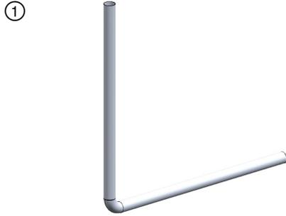
As an alternative to gore segments for 2 in. and smaller, tight bend radius elbows. Hilti Endo-Shield may be wrapped around the straight sections of pipe adjacent to the elbow per individual layers or continuous wrapping methods except material shall not be taped permanently to pipe.
