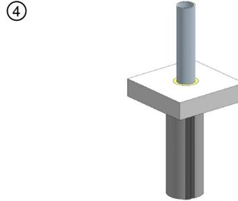
Apply 3 in. wide aluminum foil tape or FSK tape over the longitudinal seam.
