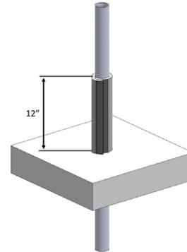
A 2 in. overlap of longitudinal seam shall be included. Apply 3 in. wide aluminum foil tape or FSK tape over the longitudinal seam. For 1 hr. T-rating, one layer of pipe covering shall be continuously wrapped around the penetrant, extending min 12 in. (305 mm) above the floor.
