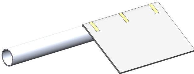
Hilti Endo-Shield may be continuously wrapped around the conduit. Using min 1/2 in. wide filament tape, FSK tape or aluminum foil tape, attach leading edge of Hilti Endo-Shield onto the conduit and wrap continuously.
