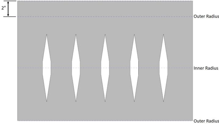
The elbows are each fitted with a gore segment cut to accommodate the elbow radius that occurs as the Hilti Endo-Shield is wrapped radially around the elbow.
