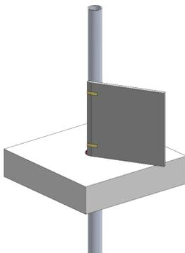
Layer 1: Tape Hilti Endo-Shield to the conduit with min. 1/2 in. wide filament tape, FSK tape or aluminum tape.
