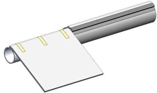
Wrap adjacent section continuously per previous instructions. Additional wrap sections are added to insulate all straight runs of tubing.
