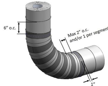
At the elbow space steel tie wire at max 2 in. on center and centered on the interior radius of each individual segment.
