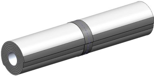
The radial seams are butted end to end without overlap. Apply 3 in. wide aluminum foil tape or FSK tape over the seam and overlap 2 in. back onto itself.
