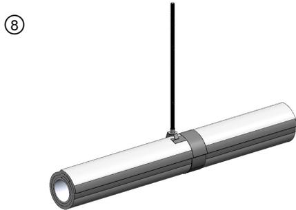
Apply 3 in. wide aluminum foil tape or FSK tape over the radial seam and overlap 2 in. onto itself. Add a piece of aluminum foil tape or FSK tape over relief cut.
