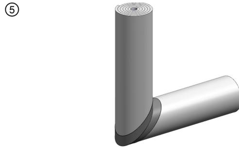
Apply 3 in. wide aluminum or FSK tape over the seam of the adjoining pieces of Hilti Endo-Shield.
