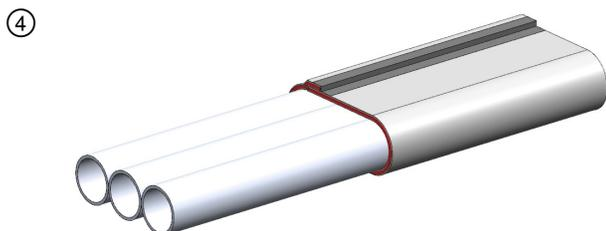
Prior to installing the adjacent section, apply 1/8 in. wet thickness of Hilti CP 606 or FS-ONE MAX over the entire edge of Hilti Endo-Shield Layer 1.
