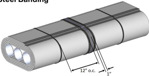
Secure final wrap with 1/2 in. wide stainless-steel banding located 1 in. from each radial seam. Space the steel banding 12 in. on center between seams.
