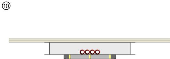
Hilti FS-ONE MAX or CP 618 Firestop Putty to fill circular cutouts made to accommodate pipes, tubes, or conduits.
