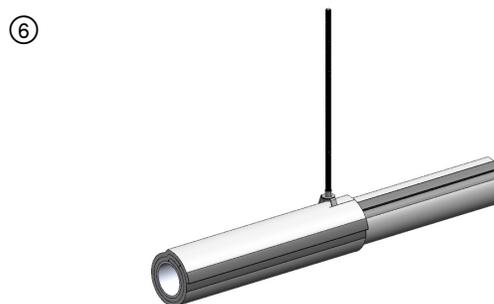
Wrap second layer of Hilti Endo-Shield in the same manner as Layer 1. The start of Layer 2 begins at the longitudinal seam of Layer 1, secured with 3 in. wide aluminum foil tape or FSK tape covering the full length of the seam. Radial seams can be treated in accordance with any of the seam methods outlined on the installation instructions for straight runs.
