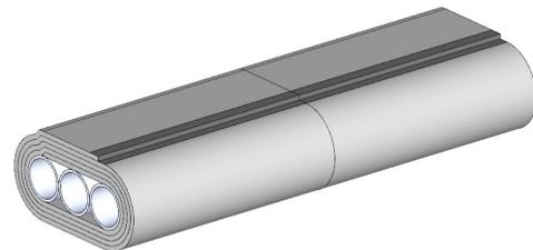
Wrap Hilti Endo-Shield continuously adding the number of layers required by manufacturer. A 2 in. overlap of longitudinal seam shall be included for each layer required. For example, a 4-layer system requires an 8 in. overlap on a final layer. Apply 3 in. wide aluminum foil tape or FSK tape over the longitudinal seam.
