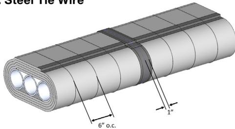
Secure outer layer with min 18 GA steel tie wire located 1 in. from each radial seam. Space the steel tie wire 6 in. on center between the seam.
