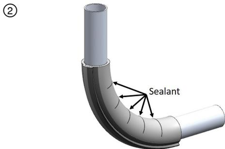
Attach Layer 1 using min 1/2 in. wide filament tape, FSK tape or aluminum foil tape. Fill all gore segment seams with 1/8 in. thick of Hilti CP 606 or FS ONE MAX. Wrap Hilti Endo-Shield tightly around the tubing overlapping 2 in. at the longitudinal seam. Apply 3 in. wide aluminum foil tape or FSK tape over the longitudinal seam.
