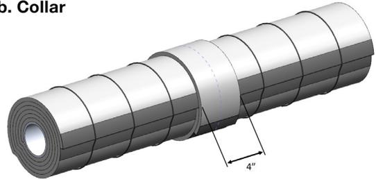
At radial seams and seams between the gore end segment and adjoining straight section, add an additional 4 in. wide section of Hilti Endo-Shield. It may be centered over the radial seam of the final layer overlapping 2 in. at the longitudinal seam. Apply 3 in. wide aluminum foil tape or FSK tape over the longitudinal seam of the 4 in. wide section of Hilti Endo-Shield. Secure with Steel tie wire.
