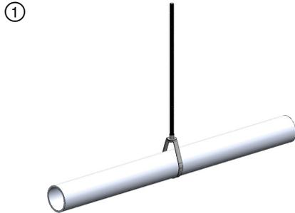
Traditionally critical conduits are supported with swivel loop hangers as shown in the picture above.
