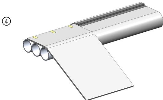
Install adjacent wrapped section as per previous instructions. Additional wrapped sections are added to insulate all straight runs of tubing.
