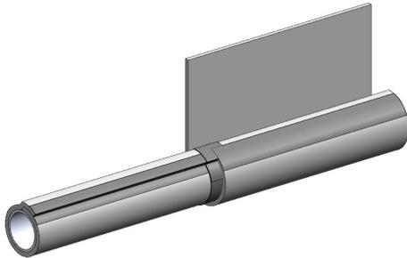
Layer 2: Wrap second layer of Hilti Endo-Shield in the same manner as Layer 1. The start of Layer 2 begins at the longitudinal seam of Layer 1, secured with 3 in aluminum foil tape or FSK tape covering the full length of the seam.
