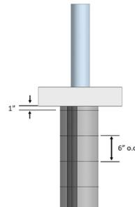
Wrap min 18 GA Steel tie wire, 1 in. from concrete interface and 6 in. on center steel tie wire spacing.
