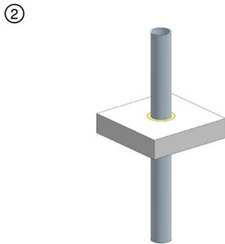
Min 4 in. (102 mm) thickness of min 4 pcf (64 kg/m<sup>3</sup>) mineral wool batt insulation firmly packed into annular space between pipe and opening as a permanent form. Packing material to be installed flush with bottom of floor and recessed from top surface of floor or from both surfaces of wall to accommodate the required thickness of fill material.
