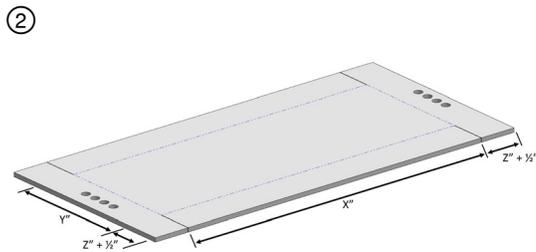
One layer sized to cover back and four sides of steel box. Add relief cuts per box side dimensions. Circular openings made in wrap material to accommodate pipes, tubes or conduits sized max 1/2 in. (13 mm) larger than the outside diameter of the pipe, tube, or conduit.
