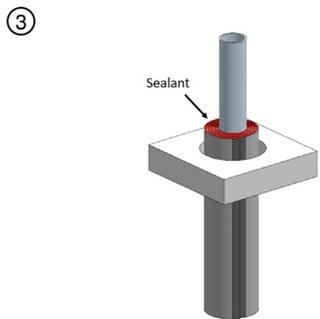
Apply 1/8 in. thick depth of Hilti CP 606 or FS-ONE MAX to be applied to cover edge section.
