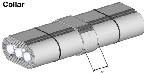
At radial seams and seams between the elbow end segment and adjoining straight section, add an additional 4 in. wide section of Hilti Endo-Shield. Center over the radial seam of the final layer overlapping 2 in. at the longitudinal seam. Apply 3 in. wide aluminum foil tape or FSK tape over the longitudinal seam of the 4 in. wide section of Hilti Endo-Shield. Secure with Steel banding per 9a.
