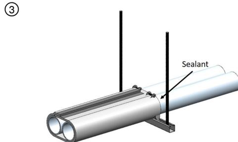
Apply 1/8 in. wet thickness Hilti CP 606 or FS-ONE MAX to the relief cuts and Layer 1 edge as shown on the picture. Apply 3 in. wide aluminum foil tape or FSK tape over the longitudinal seam.
