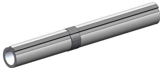
The radial seams are butted end to end without overlap. Apply 3 in. wide aluminum foil tape or FSK tape over the seam and overlap 2 in. back onto itself.
