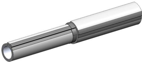
Tightly wrap Layer 2 over Layer 1 and overlap the longitudinal seam by 2 in. Cover the full length of the longitudinal seam with 3 in. wide aluminum foil tape or FSK tape.
