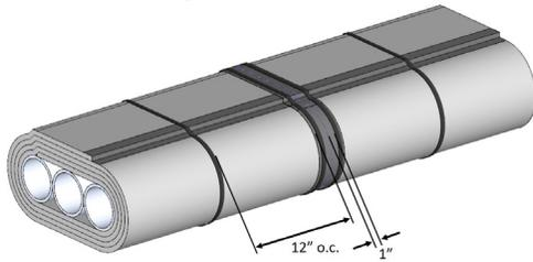
Secure outer layer with 1/2 in. wide stainless-steel banding located 1 in. from each radial seam. Space the steel banding 12 in. on center.
