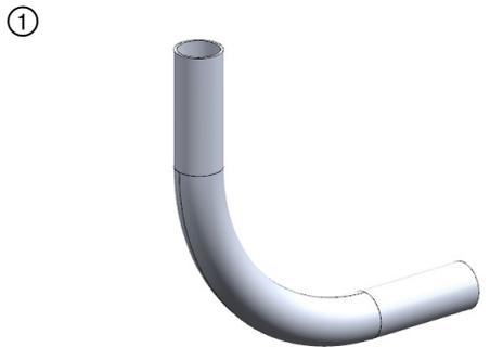
Start Layer 1 at the outermost radius of the elbow
