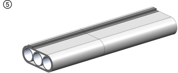
Apply 3 in. wide aluminum foil tape or FSK tape over the longitudinal seam.
