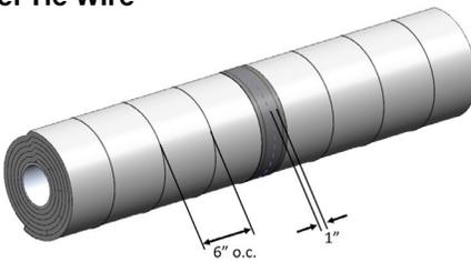
The outer layer is secured with min 18 GA steel tie wire located 1 in. from each radial seam. Space the steel tie wire 6 in. on center between the seam.
