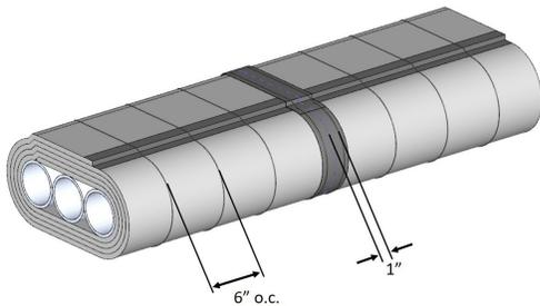
Secure final wrap with min 18 GA steel tie wire located 1 in. from each radial seam. Space the steel tie wire 6 in. on center between the seam.
