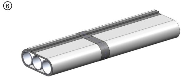
The radial seams are butted end to end without overlap. Apply 3 in. wide aluminum foil tape or FSK tape over the seam and overlap 2 in. onto itself.
