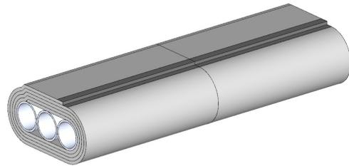
Hilti Endo-Shield may be continuously wrapped around the conduit bank. Using min 1/2 in. wide filament tape, FSK tape or aluminum foil tape, attach leading edge of Hilti Endo-Shield onto the conduit and wrap continuously.
