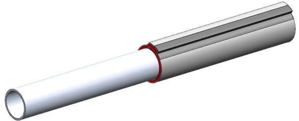
Add 1/8 in. depth of Hilti CP 606 or FS-ONE MAX at the edge of first layer. Ensure compatibility with piping material.
