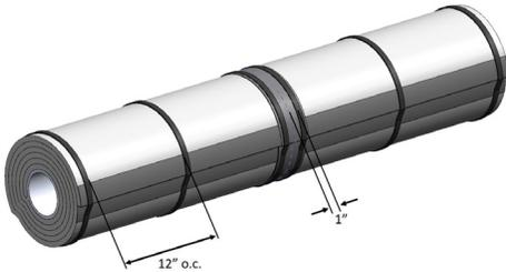
The outer layer is secured with 1/2 in. wide stainless-steel banding located 1 in. from each radial seam. Space the steel banding 12 in. on center.
