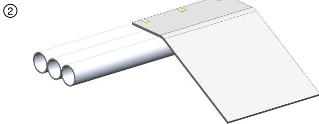
Layer 1: Tape Endo-Shield to the conduit with min 1/2 in. wide filament tape, FSK tape or aluminum foil tape.
