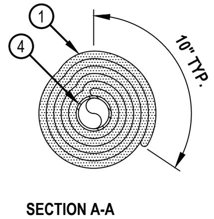
Figure 1. Min. 3 in. Steel Pipe, 5 Layers of Hilti Endo-Shield Specifications - Outer Containment Pipe Only Shown
