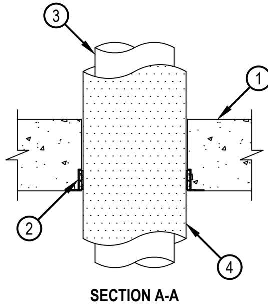
1. Floor Assembly — Min 4-1/2 in. (114 mm) thick reinforced lightweight or normal weight (100-150 pcf or 1600-2400 kg/m<sup>3</sup>) concrete floor.
