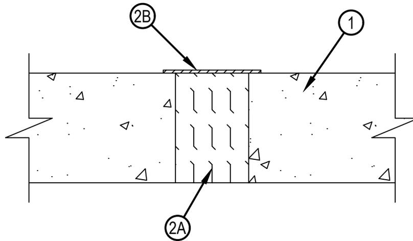
1. Floor Assembly — Min 4-1/2 in. (114 mm) thick reinforced lightweight or normal weight (100-150 pcf or 1600-2400 kg/m<sup>3</sup>) structural concrete.
