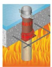
Installed CP 680 with standoff component
