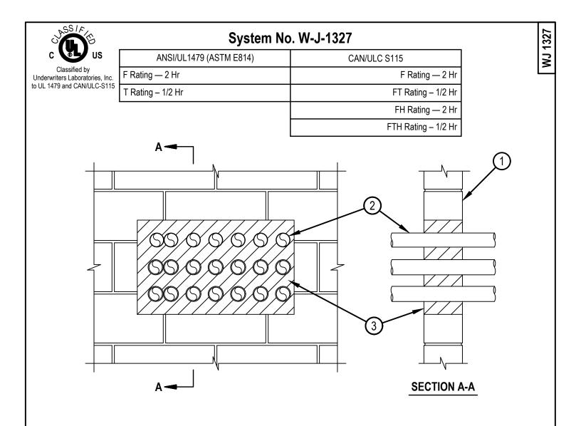
1. Wall Assembly —Min 6 in. (152 mm) thick reinforced lightweight or normal weight (100-150 pcf or 1600 - 2400 kg/m3) concrete wall. Wall may also be constructed of any UL Classified Concrete Blocks\*. Max area of opening is 360 in2 (2323 cm2) with max dimension of 24-1/2 in. (622 mm).
